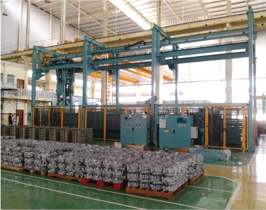
A batch of components being impregnated on a fully automatic IMPREGSEAL machine
